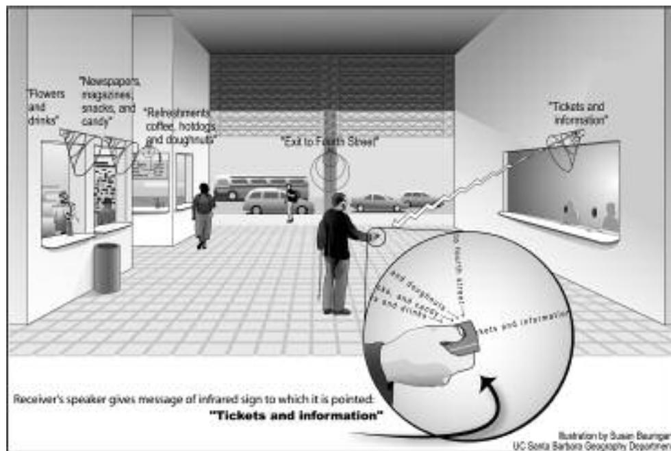
**Figure 11 - A Schematic of the RIAS System**
